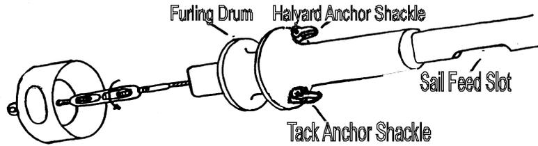
11. Slide the furling drum over the luff with the sail feed slot on the same side as the tack anchor shackle (see drawing above). You may knock the thrust washer (part "M" on page 2) out of place doing this. You can push the washer up into the cavity of the furling drum again. The washer is designed to ride between the furling drum and the bearing.
