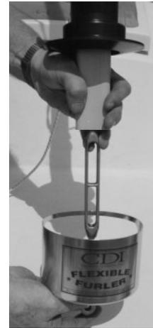
13. Pass the furling line through the hole in the side of the cup, then up through the hole in the top of the furling drum flange. Tie an overhand knot to prevent it from escaping.
