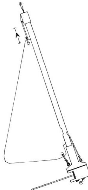
Note: When the sail is UP, the ferrule (little metal tube swaged on halyard) is DOWN near the spool.
